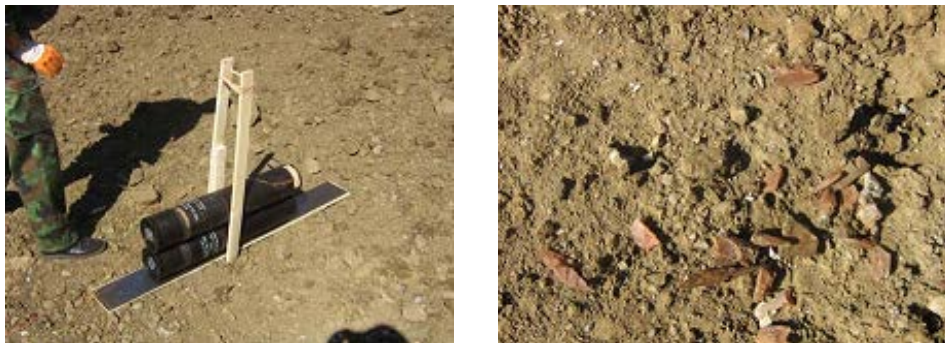
Figure 2: Sympathetic detonation test set up and detonation test result with single packaged rockets 128 mm HE WHD M63
