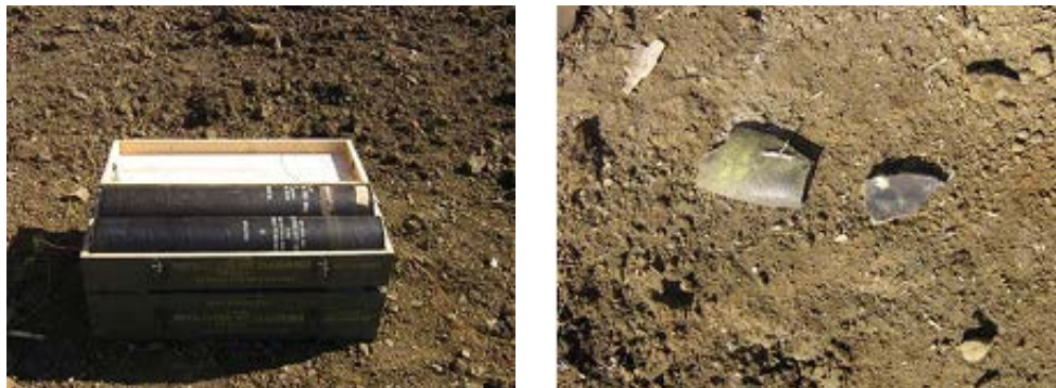
Figure 3: Sympathetic detonation test set up and detonation test result with crate packaged rockets 128 mm HE WHD M63
