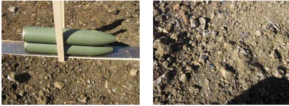
Figure 1: Sympathetic detonation test set up and detonation test result with non-packaged rockets 128 mm HE WHD M63
